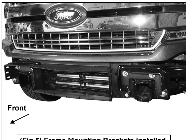
(Fig 5) Frame Mounting Brackets installed
