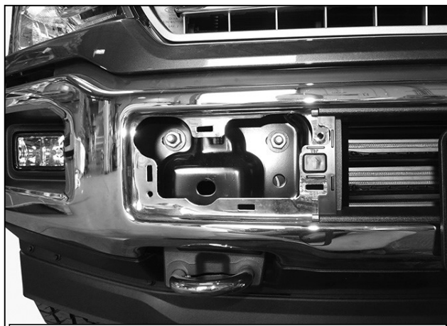
(Fig 2) Remove license plate and plastic bumper pads from bumper (passenger/right side pictured)
