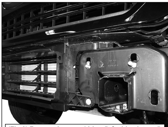
(Fig 3) Remove bumper (driver/left side pictured)
