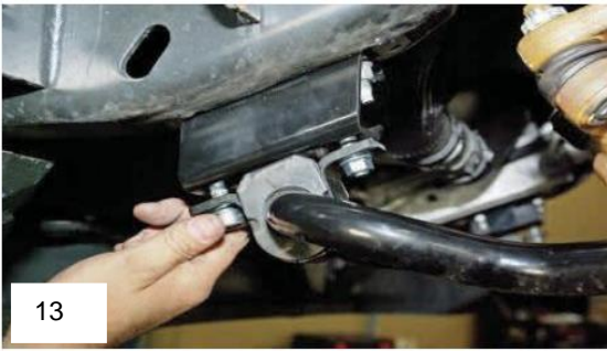
Reattached Sway bar to drop bracket using factory hardware
