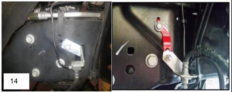
05-08 Drill a 3/8" hole 1.5" lower on the frame rail and secure brake line with original bolt. 2010-17 Reinstall brake line brackets, driver on pass side, pass on driver side. Loosen the hard line ferrule and rotate 180 degrees and retighten. Reattach brake line block to bracket with factory clips.
