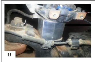
Place billet spacer on axle under spring perch.
