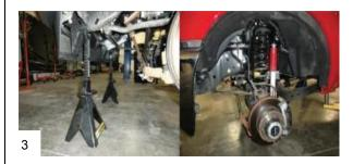
Lift front of vehicle and support with min. 3 ton jack stands. Remove front wheels and tires.
