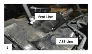
Note differential vent line and ABS brake lines and do not over stretch when lowering axle.
