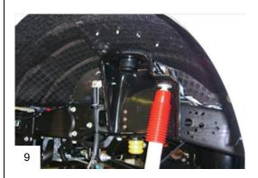
Carefully lower front axle and remove front coil springs.
