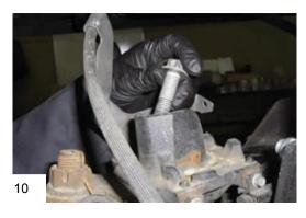
Remove bolt from middle of spring perch.
