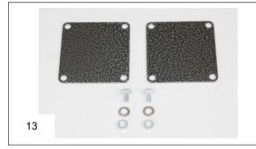
Remove the two 6mm bolts holding the ABS sensor line to the spring perch plate and install drop down bracket provided using the new 6mm bolts. Use the factory 6mm bolts and supplied washer and nuts to attach the ABS sensor line to the new drop down bracket.
