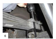
Raise axle, install new U-bolts and hardware, and tighten.
