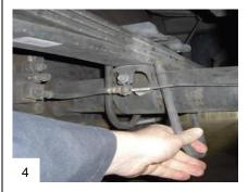
Remove U-bolts and carefully lower axle.
