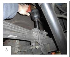
Work on one side of vehicle at a time, remove rear U-bolts.
