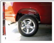
Raise and support rear frame of vehicle on level ground.
