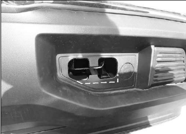
(Fig 3) Tow hook removed. Opening may need to be trimmed to clear the Mounting Bracket assembly
