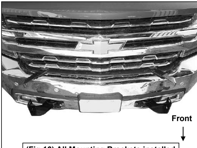
(Fig 16) All Mounting Brackets installed
