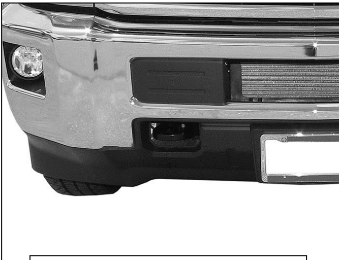
(Fig 1) Opening for tow hook pictured
