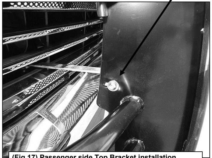
(Fig 17) Passenger side Top Bracket installation pictured. Adjust position so that Bracket cannot come in contact with plastic grille
