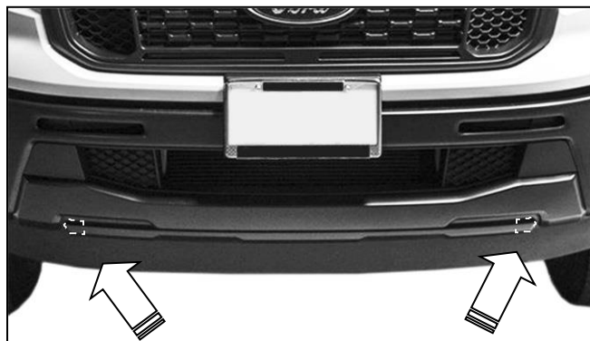
(Fig 3) Models with steel skid plate, temporarily remove skid plate to access tow hooks
