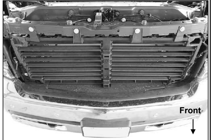
(Fig 13) Remove screws attaching grille and carefully pull grille straight out to remove grille
