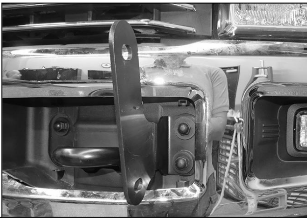
(Fig 5) Reuse factory bumper bolts to attach driver/left Frame Bracket to bumper
