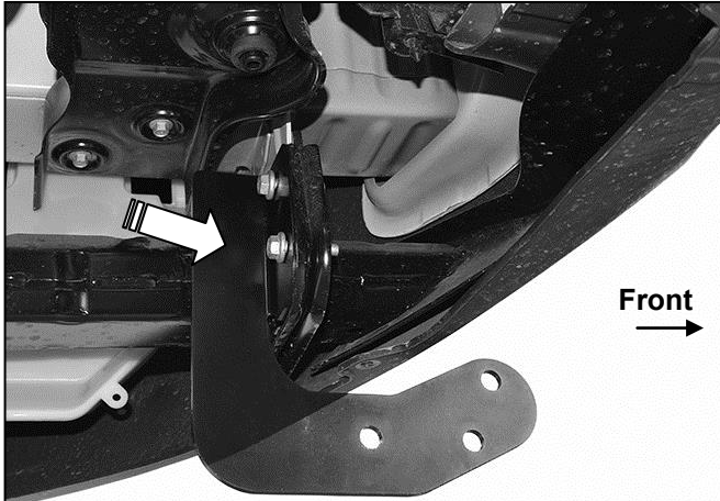
(Fig 6B) Use 12mm x 32mm Large Flat Washer for a spacer on lower mounting bolt only between Mounting Bracket and bumper bracket (Driver side Bracket installation pictured)
