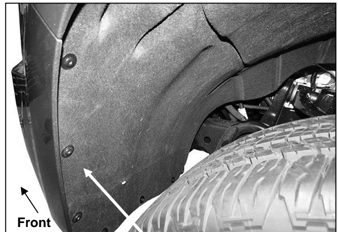
(Fig 2C) Remove hardware attaching fender liner to bumper cover
