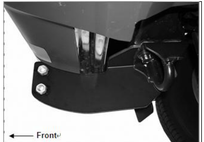
(Fig 8B) Install Frame Bracket with factory tow hook bolts. Small tow hook pictured
