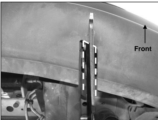
(Fig 12) Driver side Bracket installation pictured from below bumper cover. Cut cover as necessary to clear Brackets
