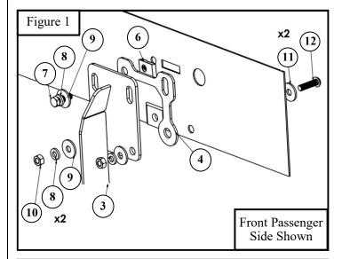
Start at the front passenger side of vehicle and grab a Mount Bracket. Use supplied M8 hardware to loosely mount the front mount bracket to the rocker panel. See Figure 1.
