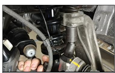
Remove the upper ball joint from the knuckle. Let knuckle hang out of the way. Do not stretch the ABS/brake lines.
