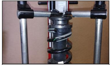
Place strut in a spring compressor. Remove factory top hat. Install in between the top hat with rubber isolator and the factory plastic spring mount.
