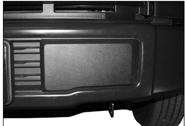
(Fig 6) Remove bumper pads to access splash guard hardware if necessary. 2015 F150 pictured
