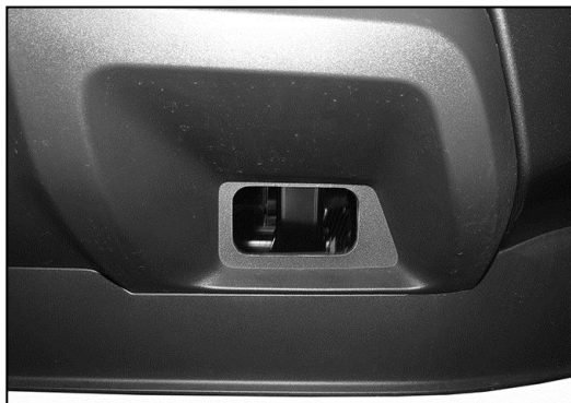
(Fig 4) Driver side after tow hook removed
