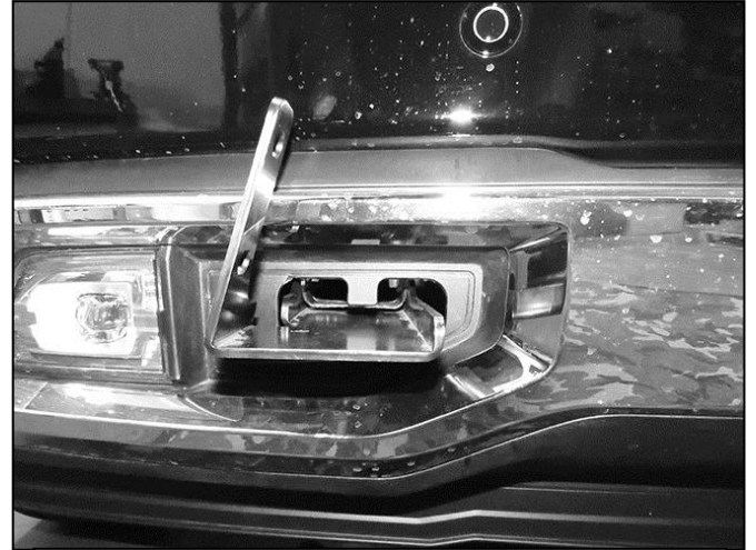
(Fig 11) Passenger/right side Bracket installed
