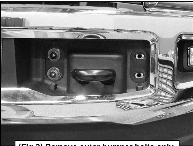
(Fig 3) Remove outer bumper bolts only (driver/left front of bumper pictured)
