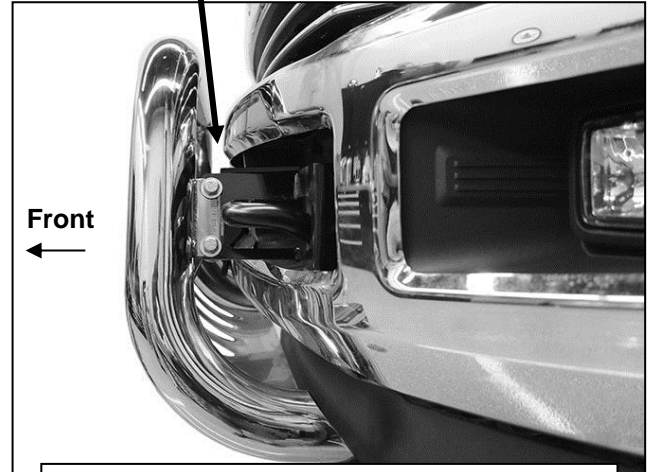
(Fig 7) Driver/left side complete installation
