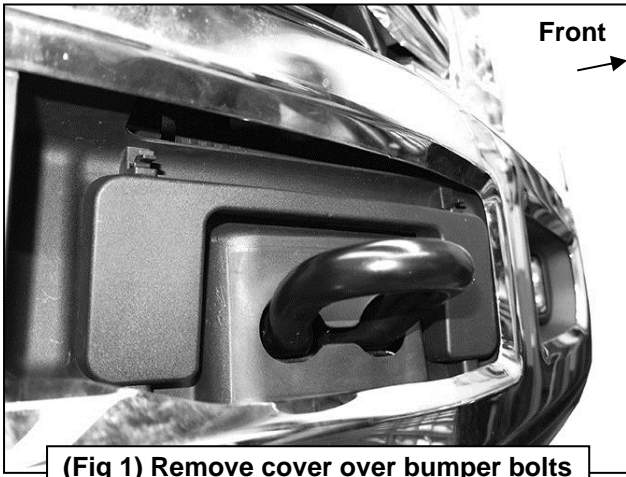
(Fig 1) Remove cover over bumper bolts
