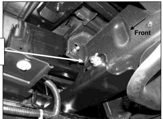
(Fig 7B) Passenger Bracket installed in "forward" position to move Bull Bar away from bumper
