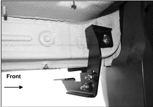
(Fig 19) Driver/left Front Bracket pictured (Note driver side front and rear Brackets are identical)
