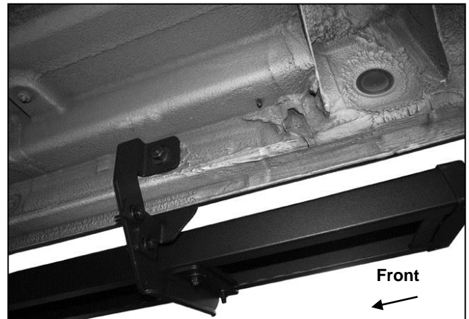
(Fig 11) Passenger side rear Bracket installed
