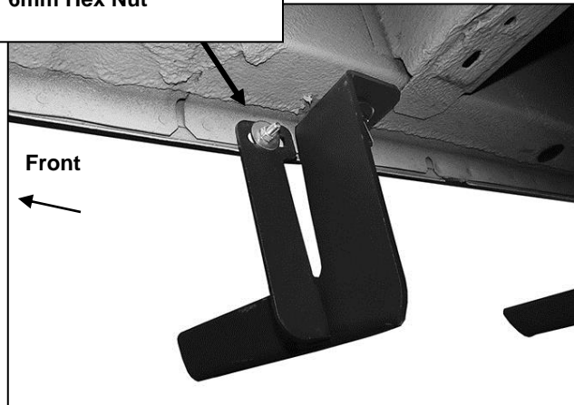
(Fig 17) Passenger/right side #2 Brackets installed
