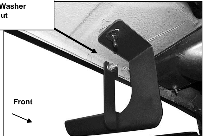
(Fig 11) Mark and drill hole through pinch weld. Attach top of Driver/left rear Support Bracket to back of pinch weld. Reinstall Running Board
