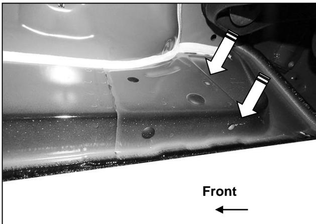
(Fig 7) Passenger/Right rear mounting location
