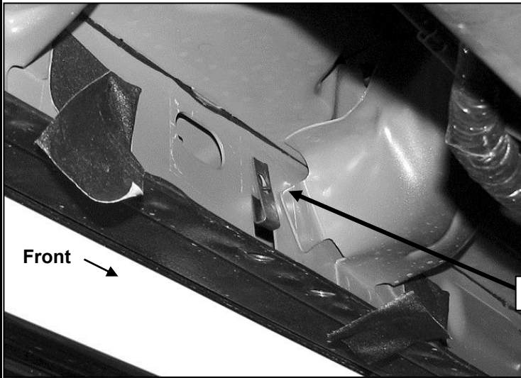
(Fig 4) Driver side-center Mounting Bracket location
