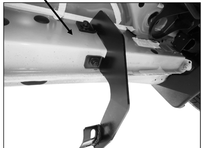
(Fig 4) Driver/left front Bracket installed
