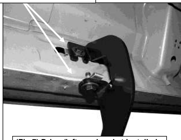
(Fig 7) Driver/left rear bracket installed
