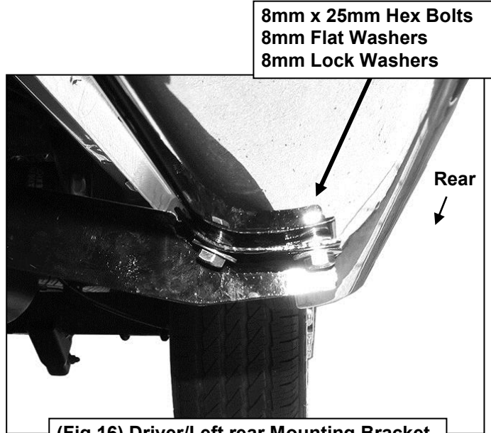
(Fig 16) Driver/Left rear Mounting Bracket
