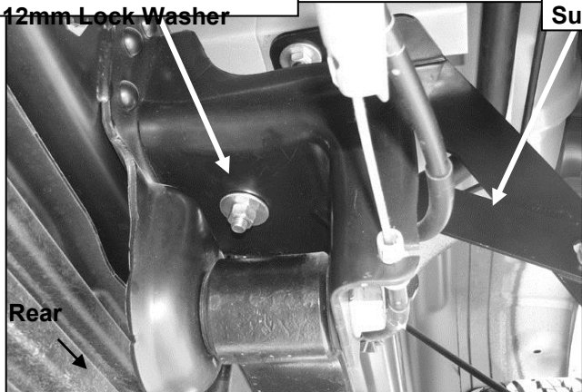
(Fig 17C) Bolt the 2011-15 driver side rear Support Bracket to the top of the rear spring mount
