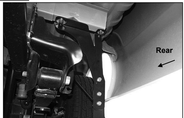
(Fig 12B) 1999-2010 Complete driver side bed Mounting Bracket assembly pictured
