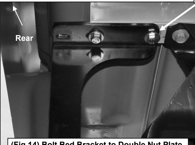
(Fig 14) Bolt Bed Bracket to Double Nut Plate
