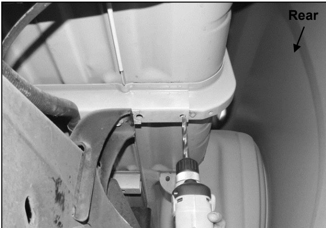
(Fig 11) Use 1/2" drill bit to open blocked off hole in bed support. Do not drill through bottom of bed
