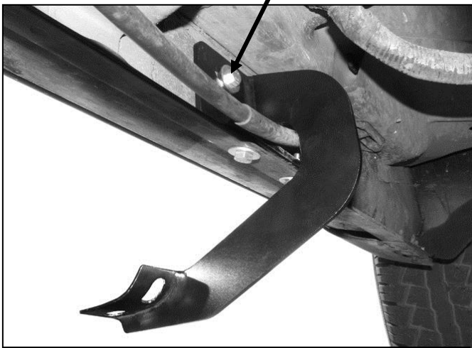
(Fig 2) Driver side-front Mounting Bracket location
