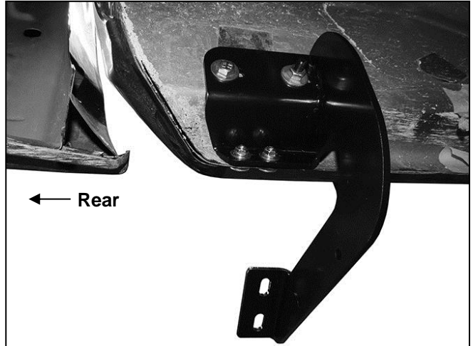
(Fig 16) Driver/Left rear Mounting Bracket assembly
