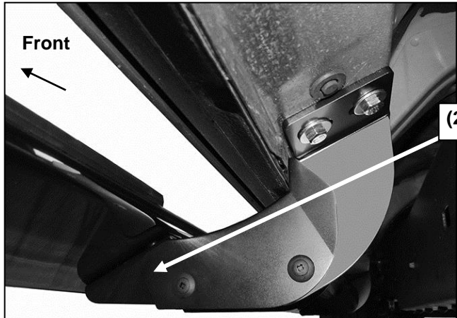
(Fig 13) Passenger center Bracket installation
