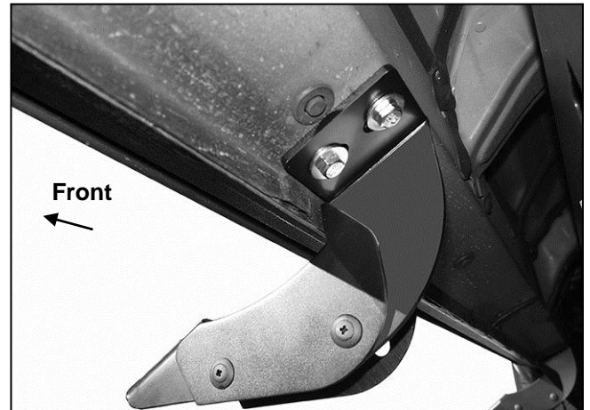
(Fig 8) Passenger side center Bracket with cover
