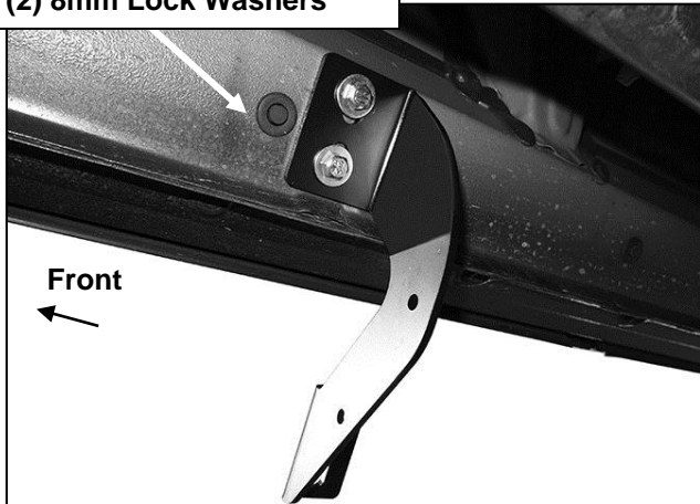
(Fig 7) Passenger side center Bracket installation
