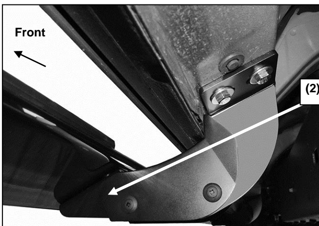
(Fig 13) Passenger center Bracket installation
