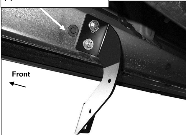
(Fig 7) Passenger side center Bracket installation
