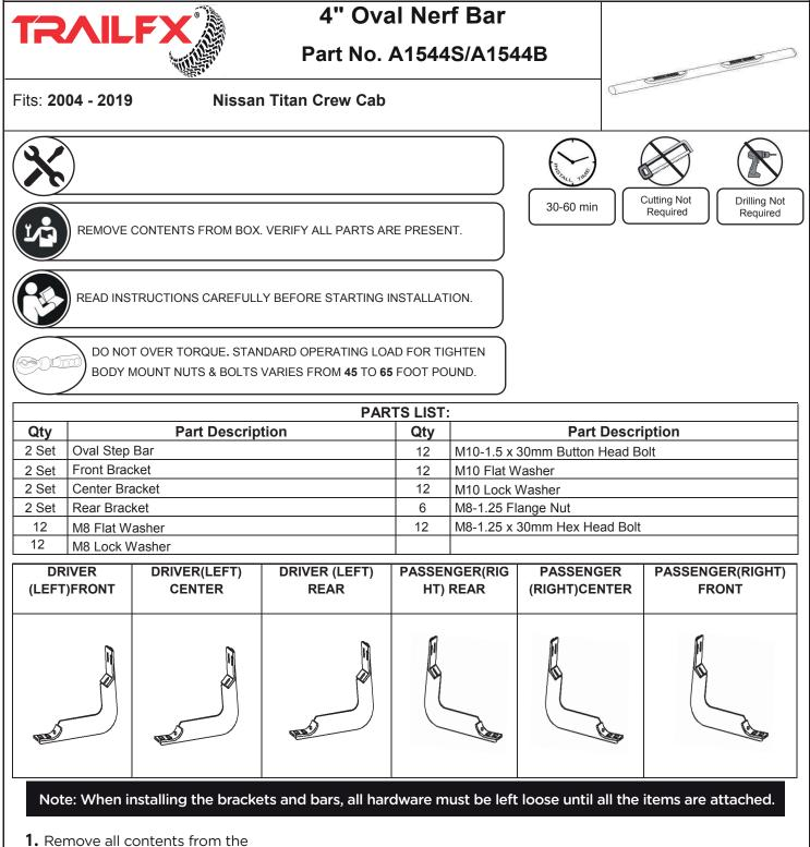
**1.** Remove all contents from the package and check stainless steel tubes for any damage. Also, verify that all components and hardware listed above are included before you begin installation.
