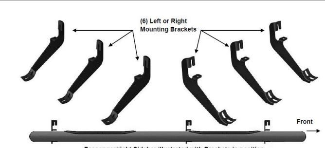
Passenger/right Sidebar illustrated with Brackets in position
