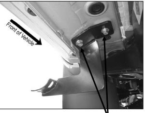
There are four sets of holes in the side panel. Starting from the front of the vehicle, use the first, second, and fourth set of holes.
