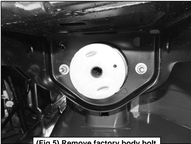
(Fig 5) Remove factory body bolt
