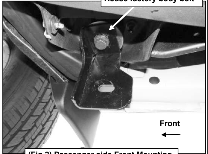
(Fig 2) Passenger side Front Mounting Bracket attached to front body mount
