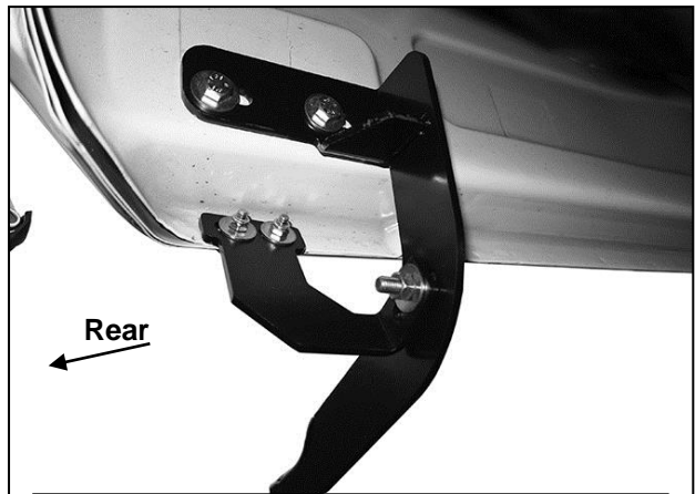
(Fig 16) Driver/Left rear Brackets installed
