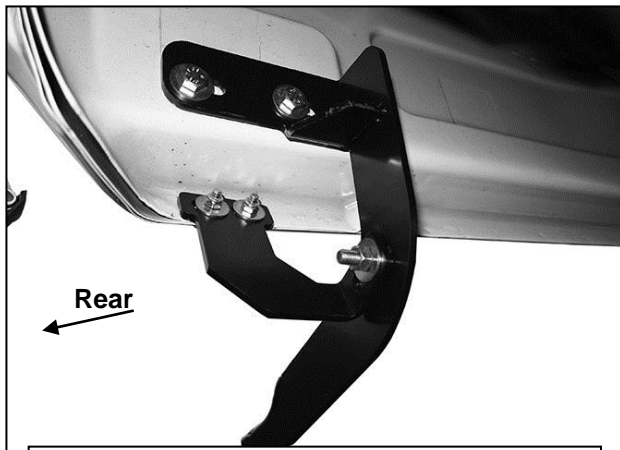
(Fig 16) Driver/Left rear Brackets installed
