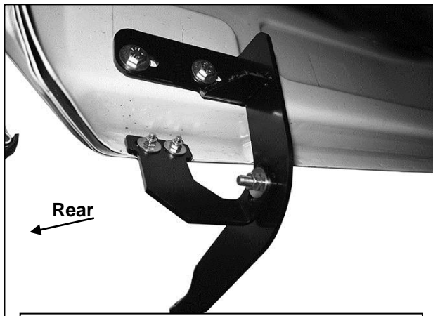
(Fig 16) Driver/Left rear Brackets installed
