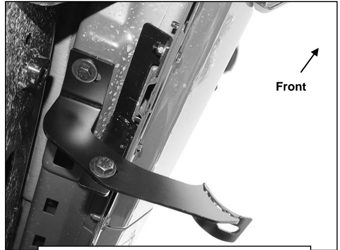
(Fig 6) Driver/left front Brackets installed
