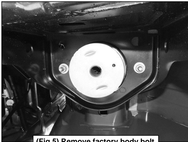
(Fig 5) Remove factory body bolt
