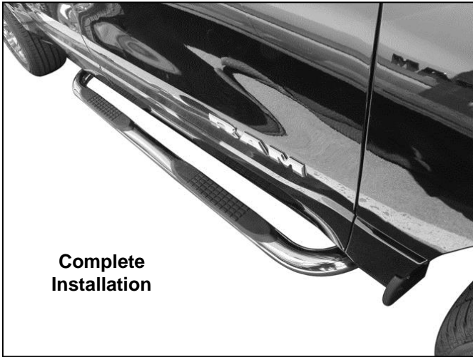
(Fig 12) Driver/left Front Brackets and Sidebar installed
