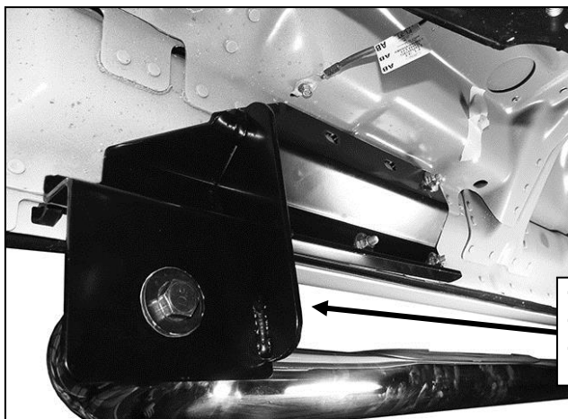
(Fig 5) Passenger side front Bracket installation
