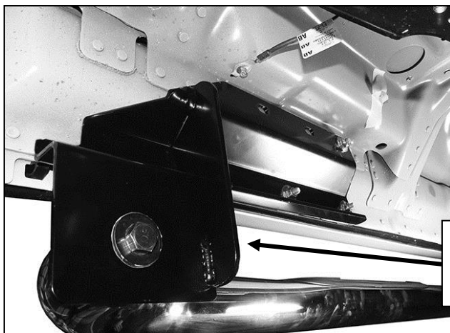
(Fig 5) Passenger side front Bracket installation
