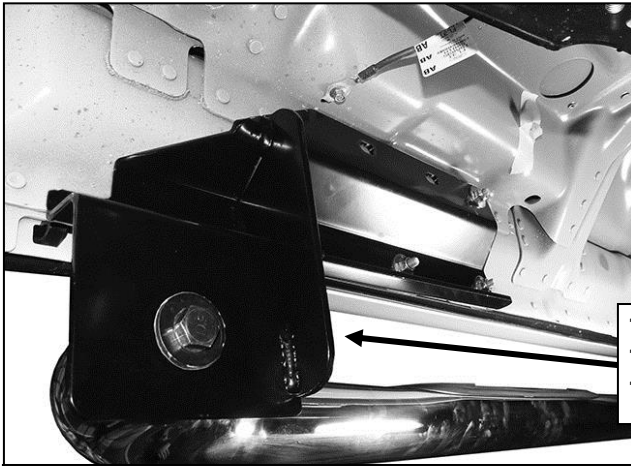
(Fig 5) Passenger side front Bracket installation
