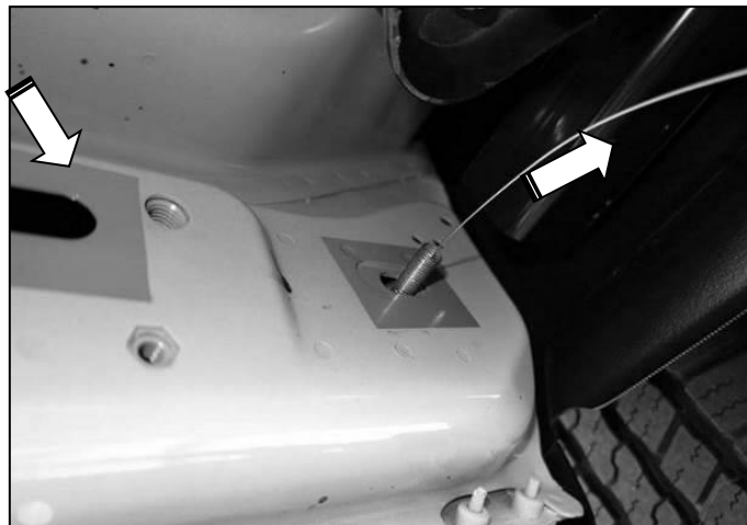
(Fig 3) With the 10mm Bolt Plate attached, slowly pull the Fish Wire back through the forward hole in the body panel. Once completely exposed as pictured, firmly hold the Bolt Plate in place, remove the Fish Wire and thread (1) 10mm Plastic Retainer onto the Bolt Plate to hold it in place (see Fig. 7A),
