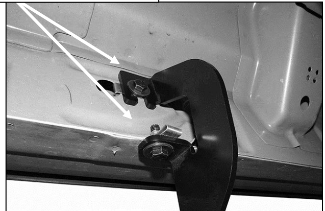
(Fig 7) Example of Bracket bolted to 8mm Clip Nuts on mounting tab and inner body panel
