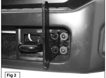
**WARNING!** Do not remove passenger and driver bumper bolts at the same time or bumper may fall. Only remove and install one Frame Mounting Bracket at a time.
