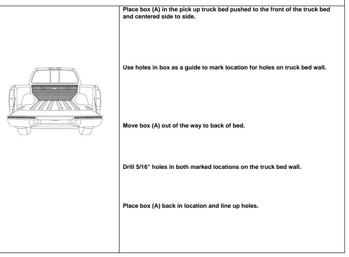
WARNING: Before drilling into your truck bed, check under your vehicle to ensure the drill location does not puncture, cut or obstruct any brake or fuel fluid lines, electrical wires, fuel tanks, etc. Mounting bolts should be installed from the underside to help prevent any damage underneath your vehicle.
